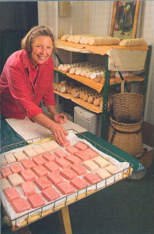
Gayl removes soaps from molds and arranges them on trays to dry and cure for 30 days.
