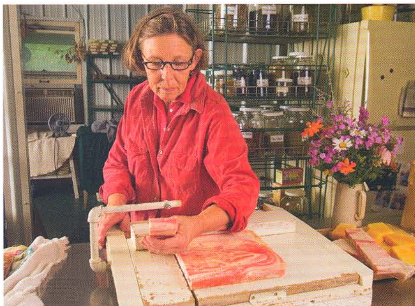
Gayl's handy, homemade cutting board employs a taut guitar string to slice through large blocks of soap, allowing her to create usable bars.
